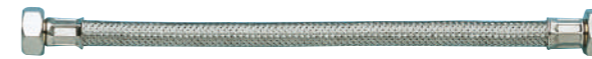
700/12 | DN8 FLESSIBILE ACCIAIO INOX 7 FILI Ø 12 3/8F X 3/8F CM 30-35-40-50-60-80-100 STAINLESS STEEL HOSE 7 WIRES Ø 12 3/8F X 3/8F CM 30-35-40-50-60-80-100
